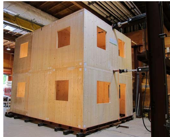
2 Storey CLT Structure Testing FPInnovations
